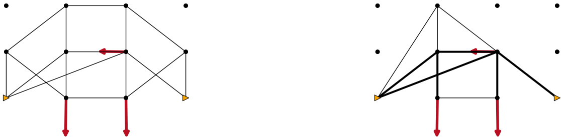
Figure 2 – Examples for bridges with twelve nodes, three different forces and 49 potential bars. In the left picture we only had to decide if a bar exists or not (b1-d1-20). On the right side, there are two different bar areas allowed (b3-d2-30).
