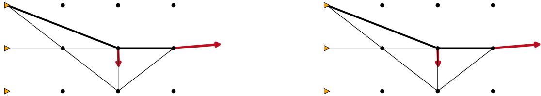
Figure 1 – Two exemplary cantilever instances with twelve nodes, two different loads and 47 potential bars. In the left picture (m2-d2-17) the maximal volume was 17, in the right one, we allowed an overall volume of 25 (m3-d2-25).
